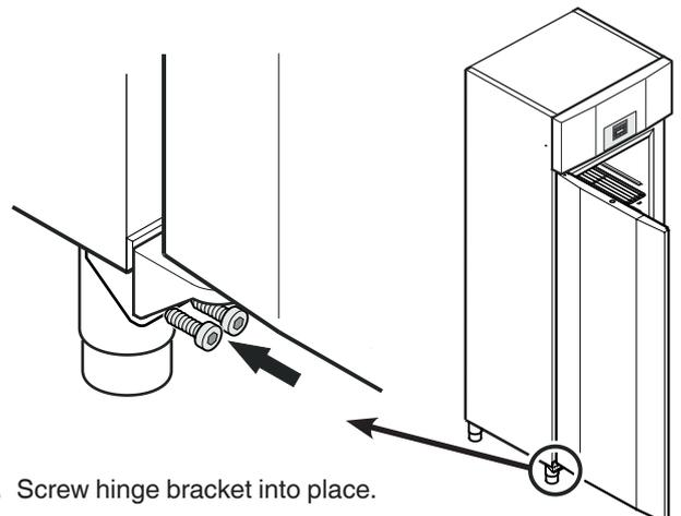
12. Screw hinge bracket into place.
