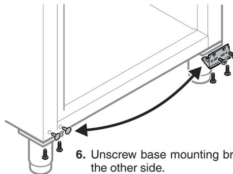
6. Unscrew base mounting bracket and attach on the other side.
