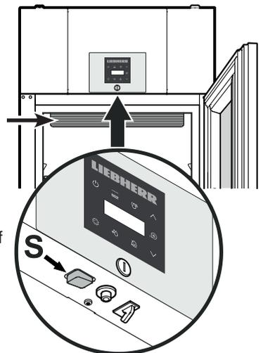
It can be switched on and off by pressing the switch S.
